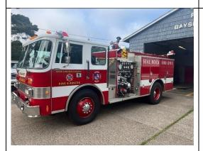
Engine E-64 1991 Pierce 700-gallon tank. 1250 GPM pump
